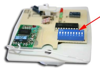
Remove 2x cross head screws and lift cover from receiver. Push up 1 or more dip switches to match Transmitter. Replace cover.
