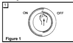
**Manual switch operation (when fitted)**: The manual switch will provide Fixed On / Timed / Fixed Off control, thereby allowing manual control of the output without disrupting the timed (tappet) settings. Please see diagram below.
