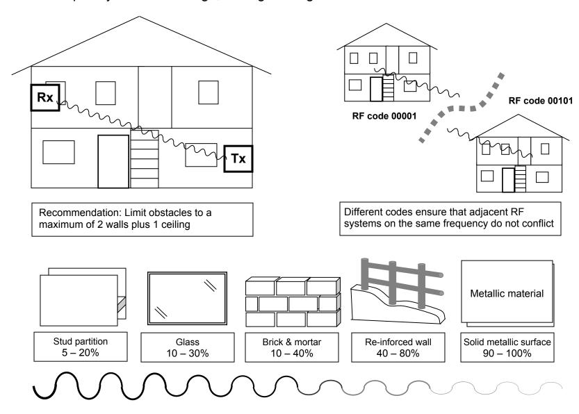
Approximate reduction in RF signal strength after passing through different materials
