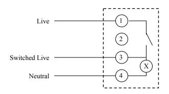
The Tower room thermostat is a bi-metal temperature regulating device. The unit is fitted with an accelerator heater to give a close differential for accuracy of temperature control. A neutral connection must be fitted and the device is only for mains operation.
