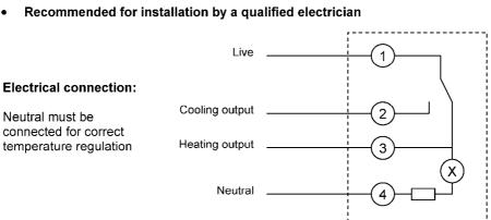
The Tower Heat-Cool thermostat is a bi-metal temperature regulating device. The unit is fitted with an accelerator heater to give a close differential for accuracy of temperature control. A neutral connection must be fitted and the device is for mains operation only.
