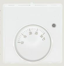
Designed for wall mounting, with 60mm fixing centres for back-box compatibility, and suitable for in-wall or surface-run wiring connection. The thermostat cover incorporates four breakouts for surface-run conduit. The temperature regulation mechanism is the well-proven sealed bellows system.
