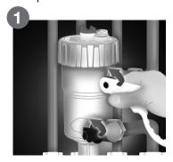
Close service valves using the spanner provided. Open the drain plug and allow the filter chamber to empty. Close drain plug.
