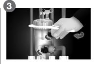
Replace the inner filter and fit a new '0' ring. Replace magnet, replace and tighten the drain plug, then open both service valves. Open bleed valve to eliminate any air in the system.
