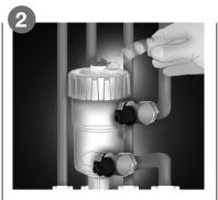
Tighten drain plug after draining and remove the bleed valve completely.
