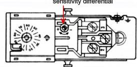
Terminal (2) = Normally Closed (Call). (Opens the circuit with increasing temperature)
