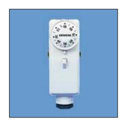
Single pole changeover thermostat with switch contacts complete with cable clamp, it is particularly suitable for measuring temperatures on heating plant pipes and Domestic hot water tanks. Thermostat clamping is achieved by means of spring-band. assuring good contact and fixing to pipe or tank surface.
