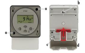
Undo the recessed cross-head screws. Grip the square timer housing and pull the timer away from the base.
