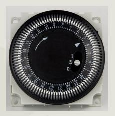
OP-FM1STUHO IS A CAPTIVE-TAPPET 24-HOUR TIME SWITCH MODULE. EACH TAPPET OP-ERATES FOR 15 MINUTES. THE TIMER IS SUITABLE FOR SUB-PANEL MOUNTING. THE 24 HOUR DIAL CONTROLS A VOLT-FREE CHANGEOVER SWITCH, WITH A RESISTIVE RATING OF 16 AMPERES. A THREE-POSITION MANUAL OVERRIDE IS BUILT-IN TO THE FACE OF THE DIAL, PROVIDING TIMED, FIX ON AND FIX OFF SELECTIONS.
