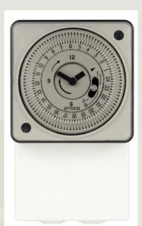
OP-IHTGPT IS A 24 HOUR IMMERSION HEATER TIME SWITCH, SUITABLE FOR SURFACE MOUNTING. THE TIMER CONTROLS A VOLT-FREE CHANGEOVER SWITCH, WITH A RESISTIVE RATING OF 16 AMPERES. PRE-FITTED (REMOVABLE) LINK FOR MAINS SWITCHING.
