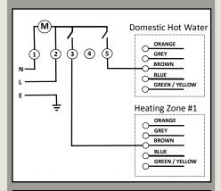
Connections for SBWF02: Controlling 1 heating zone and 1 domestic hot water using 2 x 2-port zone valves
